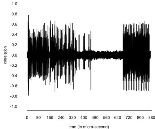
Fig. 1: Correlation between offset and power values at each time in the first round of the masked AES.
